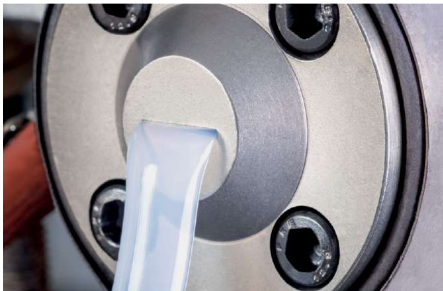
PFAS-free AddWorks PPA enhances extrusion processability (© Clariant)
